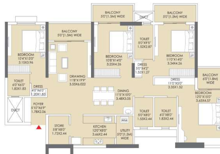
TYPICAL UNIT PLAN - 4 BHK FLAT NO. - 304 to 2004 308 to 2008
